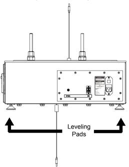
5. The Model 2006 Azimuth Positioner is configured with multiple EUT connections fitted with rotary joints to allow continuous rotation of the EUT. The maximum AC power for the slip ring is 250 VAC 10 A. Power is supplied to the system via an IEC power connection on the side of the 2006 unit. The IEC power connection includes a power filter and a non-illuminated power switch.
